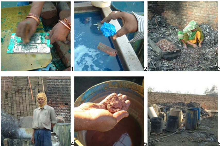
Fig. 10. The extraction of copper from printed wiring boards (PWB): (1) manually removing varnish, (2) recovering copper-sulphate after submerging PWBs for 12 h in sulphuric acid followed by boiling off H 2 O using PWB residues as a fuel, (3) manually segregating the copper layer and glass fibres after burning multi layer PWBs which are resistant to acid, (4) scrap iron is added to the remaining liquid to react with the dissolved copper, (5) fallen out copper slime is a third product bringing the total to 1 to 2 t of copper per month, (6) such an SME creates about 12 jobs, however at high external costs. (Empa Survey, 2004).
